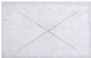
AZ150 after 240 hours of salt spray testing
